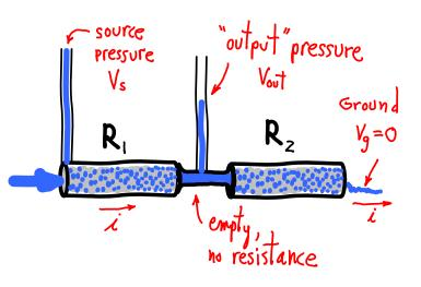
total voltage difference is  $(V_s - V_g) = V_s$  current is  $i = \frac{V_s}{(R_1 + R_2)}$
