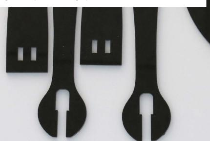
Beam deflection with scanning heads allows any complex contours that can be reprogrammed to be cut in a short time.
