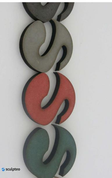
MDF stands for **Medium Density Fiberboard**. It is an engineered wood product made by breaking down hardwood or softwood residuals into wood fibres, combining it with wax and a resin binder, and forming panels. It is is generally **denser than plywood** but can be used as a building material similar in application.
