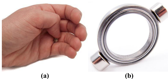
Figure 2. (a) One-handed use is more difficult, but is even more discreet. (b) We alleviate the additional friction of one-hand use by using a thin ball bearing with mounted magnets.
