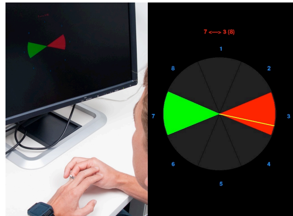
Figure 4: Participant targeting in the visual condition. The yellow pointer (in target 3) mirrors the ring's position. The target information "7 <---> 3 (8)" (indicating green target at 7, red at 3, 8 wedges total) was shown as a memory aid for the eyes-free condition.
