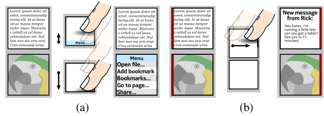
Figure 10: Proposed extensions to Facet. Image (a) shows menuing where a slight slide upwards from the bottom “pulls up” a menu; then a downward slide “pushes” the menu to the next segment. For notifications (b), a bar appears on the side of all segments. The user slides a finger from the side, and the notification appears on the segment where the touch occurred.
