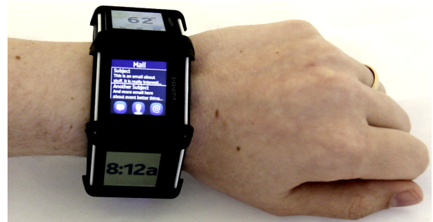
Figure 1: The Facet prototype, consisting of six WIMM One devices mounted in a bracelet such that they are removable.
