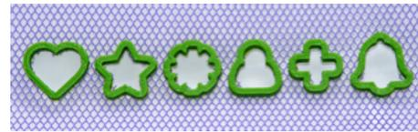
Figure 9. Arbitrarily shaped grommets 3D printed onto a polyester mesh. The centers of the grommets were cut out after printing.
