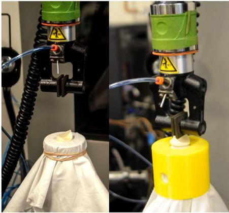
**Figure 11. Instron adhesion test setup. Left: attachment of fabric and plastic sample to test column; right: fabric anchor (yellow) with test in progress.**
