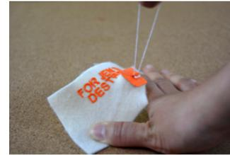
Figure 10. Plastic extruded onto a textile with a fuzzy surface creates very strong adherence. The plastic seen here is difficult to separate from a piece of felt.
