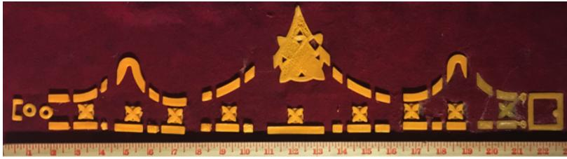
Figure 21. A 22 inch crown fabricated on a single sheet of felt by printing in rectangular sections.
