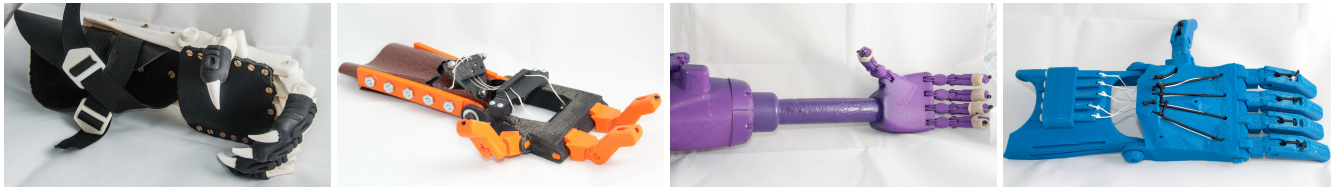
Figure 1. A variety of 3D-printed upper-limb assistive technology devices designed and produced by volunteers in the e-NABLE community. Photos were taken by the fourth author in the e-NABLE lab on RIT's campus.
